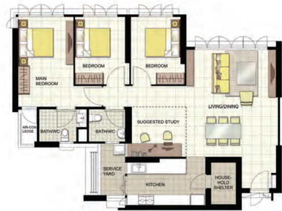
TYPICAL 5-ROOM FLOOR PLAN APPROX. FLOOR AREA 112 sqm (Inclusive of Internal Floor Area of 110 sqm and Air-Con Ledge)
