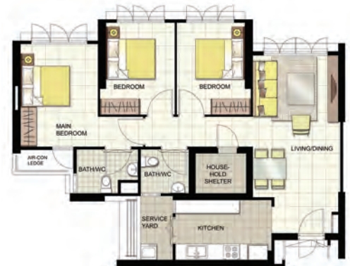
TYPICAL 4-ROOM FLOOR PLAN APPROX. FLOOR AREA 87 sqm (Inclusive of Internal Floor Area of 85 sqm and Air-Con Ledge)
