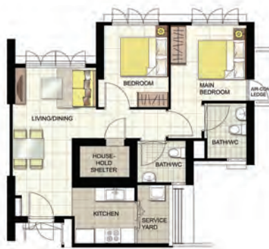
TYPICAL 3-ROOM FLOOR PLAN APPROX. FLOOR AREA 62 sqm (Inclusive of Internal Floor Area of 60 sqm and Air-Con Ledge)
