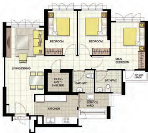
TYPICAL 4-ROOM FLOOR PLAN APPROX. FLOOR AREA 92 sqm (Inclusive of Internal Floor Area of 90 sqm and Air-Con Ledge)
