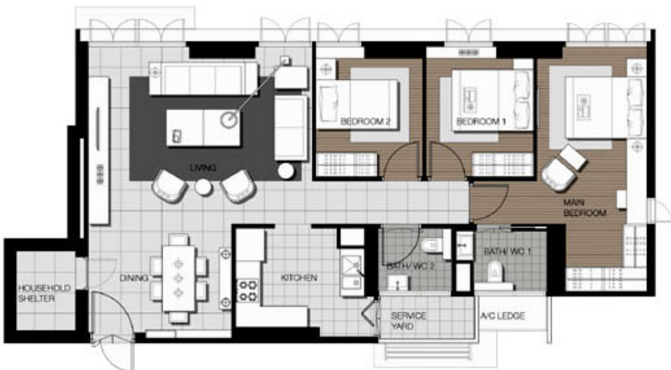
5-ROOM FLOOR PLAN APPROX. FLOOR AREA 99 sqm (Inclusive of Internal Floor Area 98 sqm and Air-Con Ledge)
