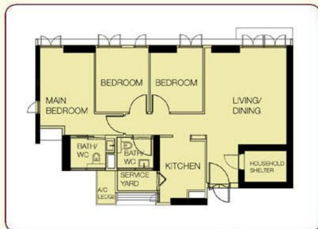
4-ROOM FLOOR PLAN APPROX. FLOOR AREA 83 sqm (Inclusive of Internal Floor Area 81 sqm and Air-con Ledge)
