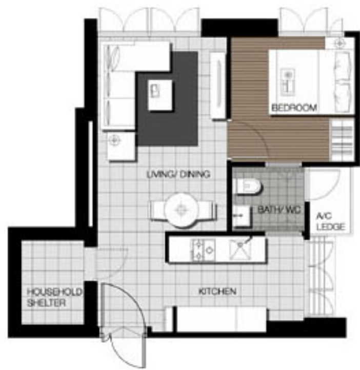
STUDIO APT FLOOR PLAN APPROX. FLOOR AREA 44 sqm (Inclusive of Internal Floor Area 42 sqm and Air-Con Ledge)
