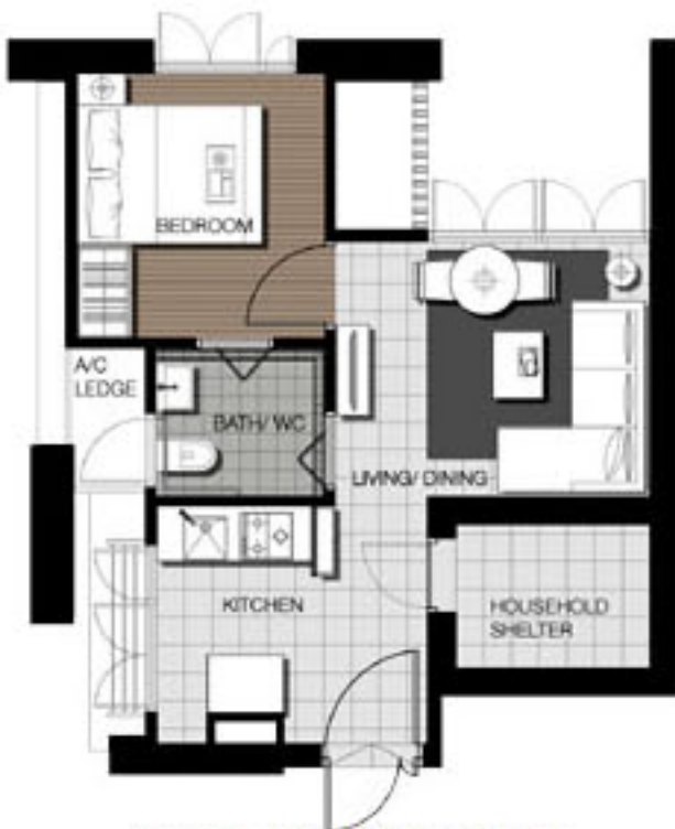
STUDIO APT FLOOR PLAN APPROX. FLOOR AREA 37 sqm (Inclusive of Internal Floor Area 35 sqm and Air-Con Ledge)
