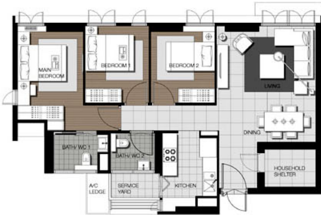
4-ROOM FLOOR PLAN APPROX. FLOOR AREA 83 sqm (Inclusive of Internal Floor Area 81 sqm and Air-Con Ledge)
