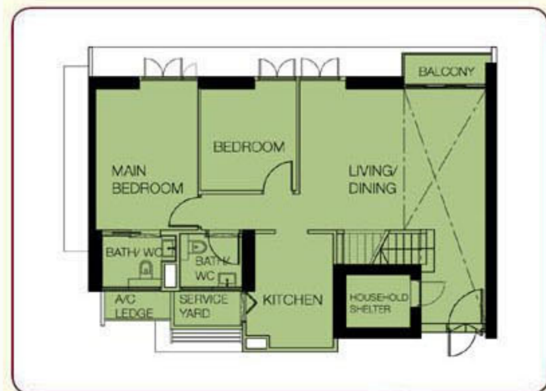
5-ROOM (LOFT 1) LOWER FLOOR PLAN APPROX. FLOOR AREA 122 sqm (Inclusive of Internal Floor Area 103 sqm, Air-con Ledge and Double Volume Space)
