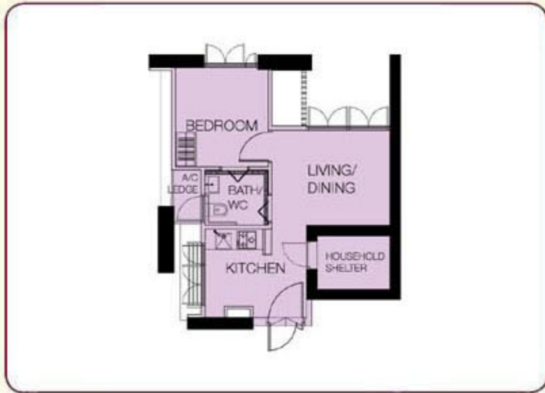
STUDIO APARTMENT FLOOR PLAN APPROX. FLOOR AREA 37 sqm (Inclusive of Internal Floor Area 35 sqm and Air-con Ledge)
