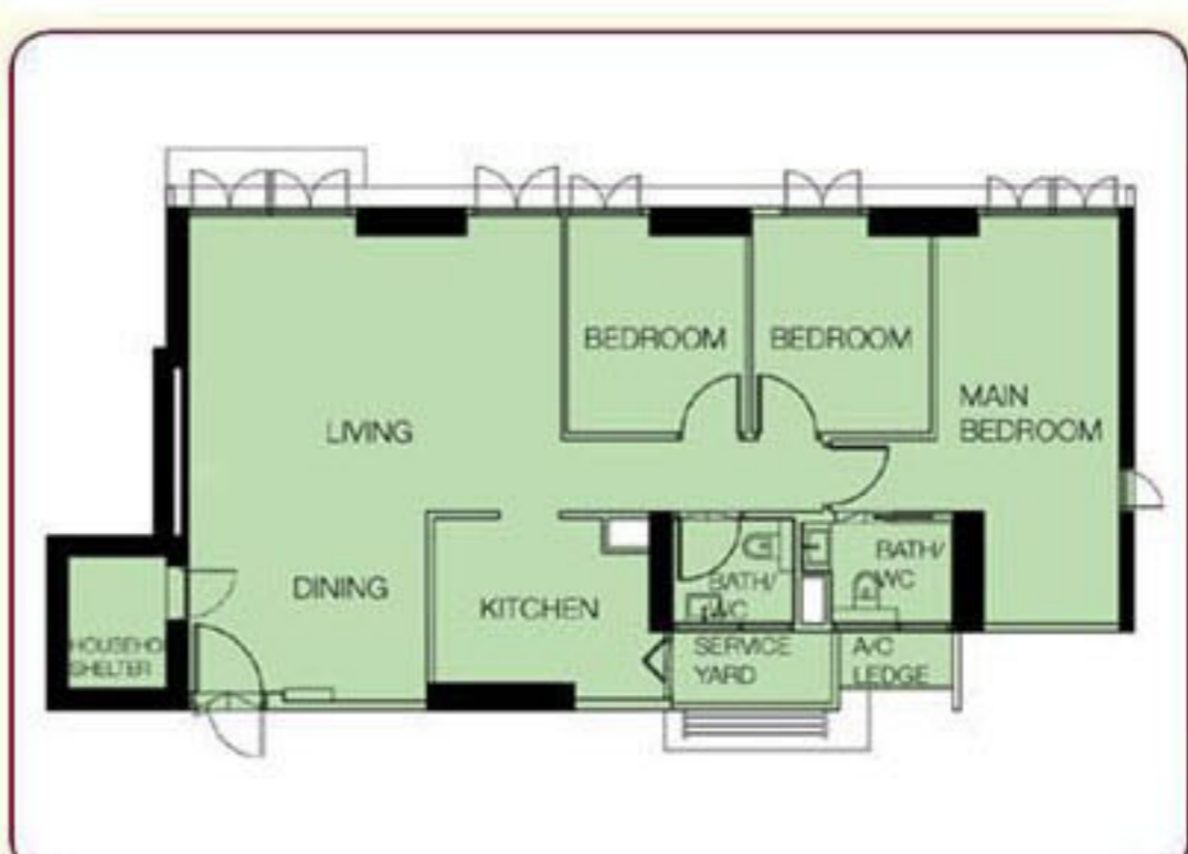
5-ROOM FLOOR PLAN APPROX. FLOOR AREA 99 sqm (Inclusive of Internal Floor Area 98 sqm and Air-con Ledge)
