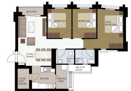
LAYOUT IDEAS FOR 4-ROOM APPROX. FLOOR AREA OF 91 sqm (Inclusive of Internal Floor Area of 88 sqm and Air-Con Ledge)
