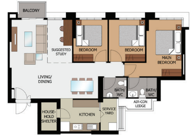
LAYOUT IDEAS FOR 5-ROOM APPROX. FLOOR AREA OF 111 sqm (Inclusive of Internal Floor Area of 108 sqm and Air-Con Ledge)
