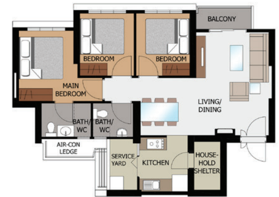
LAYOUT IDEAS FOR 4-ROOM APPROX. FLOOR AREA OF 86 sqm (Inclusive of Internal Floor Area of 83 sqm and Air-Con Ledge)
