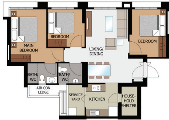
LAYOUT IDEAS FOR 4-ROOM APPROX. FLOOR AREA OF 88 sqm (Inclusive of Internal Floor Area of 85 sqm and Air-Con Ledge)
