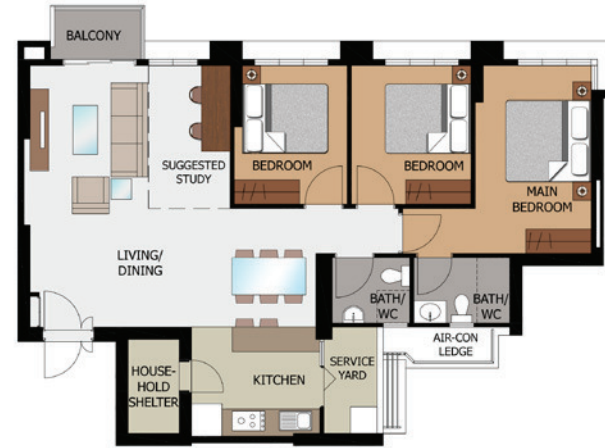
LAYOUT IDEAS FOR 5-ROOM APPROX. FLOOR AREA OF 111 sqm (Inclusive of Internal Floor Area of 108 sqm and Air-Con Ledge)
