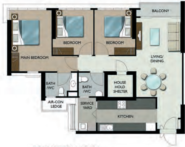
LAYOUT IDEAS FOR 4 ROOM WITH BALCONY APPROX. FLOOR AREA 98 sqm (Inclusive of Internal Floor Area 95 sqm and Air-con Ledge)
