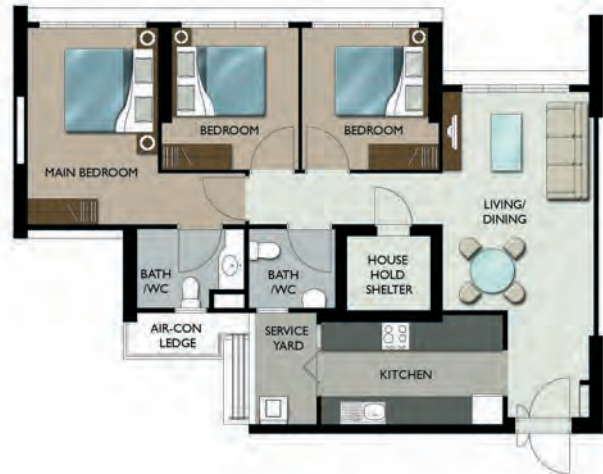
LAYOUT IDEAS FOR 4 ROOM APPROX. FLOOR AREA 88 sqm (Inclusive of Internal Floor Area 85 sqm and Air-con Ledge)
