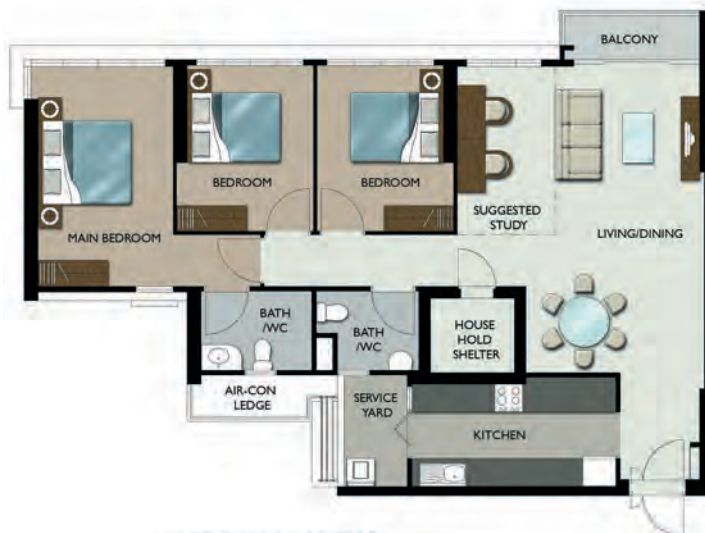
LAYOUT IDEAS FOR 5 ROOM WITH BALCONY APPROX. FLOOR AREA 116 sqm (Inclusive of Internal Floor Area 113 sqm and Air-con Ledge)
