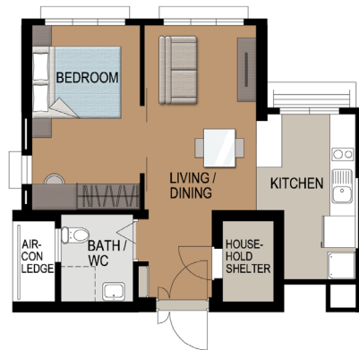
LAYOUT IDEAS FOR 2-ROOM FLEXI (TYPE 2) APPROX. FLOOR AREA OF 48 sqm (Inclusive of Internal Floor Area of 45 sqm and Air-Con Ledge)
