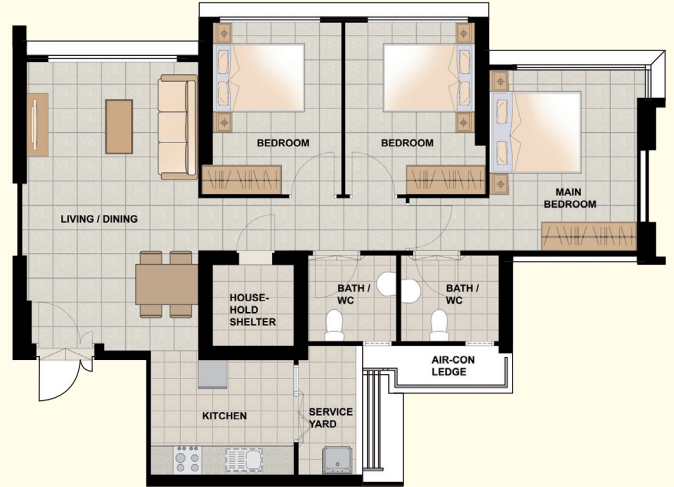
TYPICAL 4-ROOM FLOOR PLAN APPROX. FLOOR AREA 93 sqm (Inclusive of Internal Floor Area 90 sqm and Air-Con Ledge)
